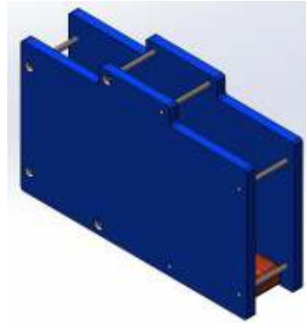
Fig. 2 Diagram of the clamp covered with insulation film
